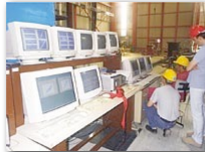
(a) physical piers in the lab, (b), schematic representation (c) workstations running the PSD algorithm and controlling the test
