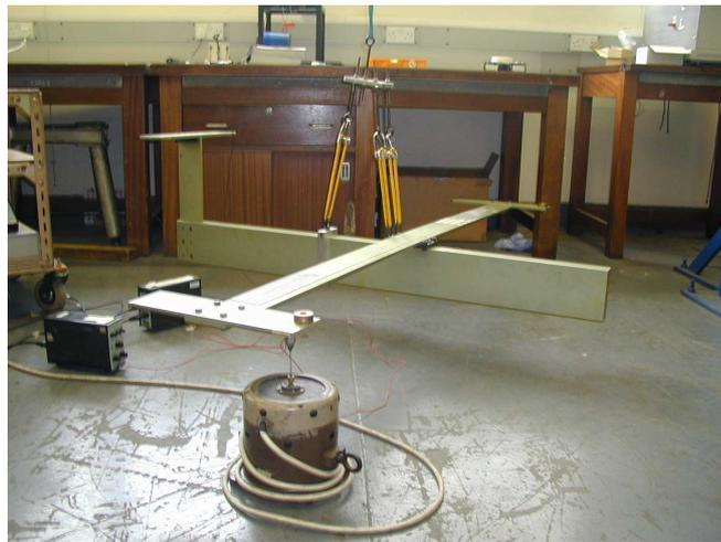
Fig. 4.12 Practical Realization - Free Structure, Fixed Exciter
