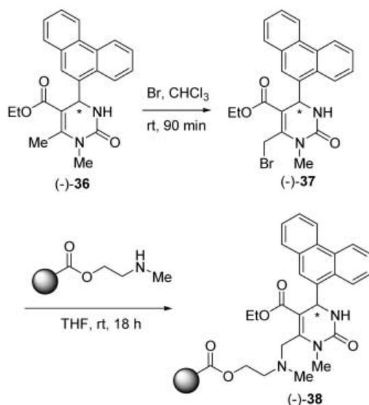
**Scheme 11.** Preparation of a DHPM-based chiral stationary phase on macroporous aminomethacrylate beads [24].
