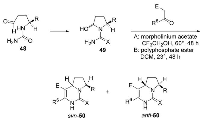
**Scheme 15.** Enantioselective intramolecular (“tethered”) Biginelli condensations for the synthesis of hexahydropyrrolo[1,2-c]pyrimidines.
