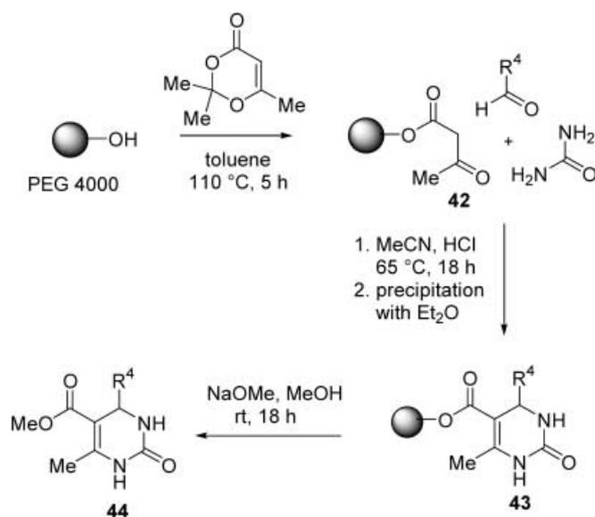
**Scheme 13.** Soluble polymer-assisted Biginelli condensation [41].
