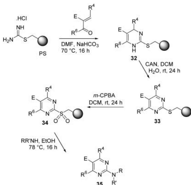
**Scheme 10.** Solid phase synthesis of 2-aminopyrimidine-5-carboxylates based on the safety-catch linker principle ( $R^4 = \text{CO}_2\text{Et}$ ,  $R^6 = \text{Ph}$ ) [36].
