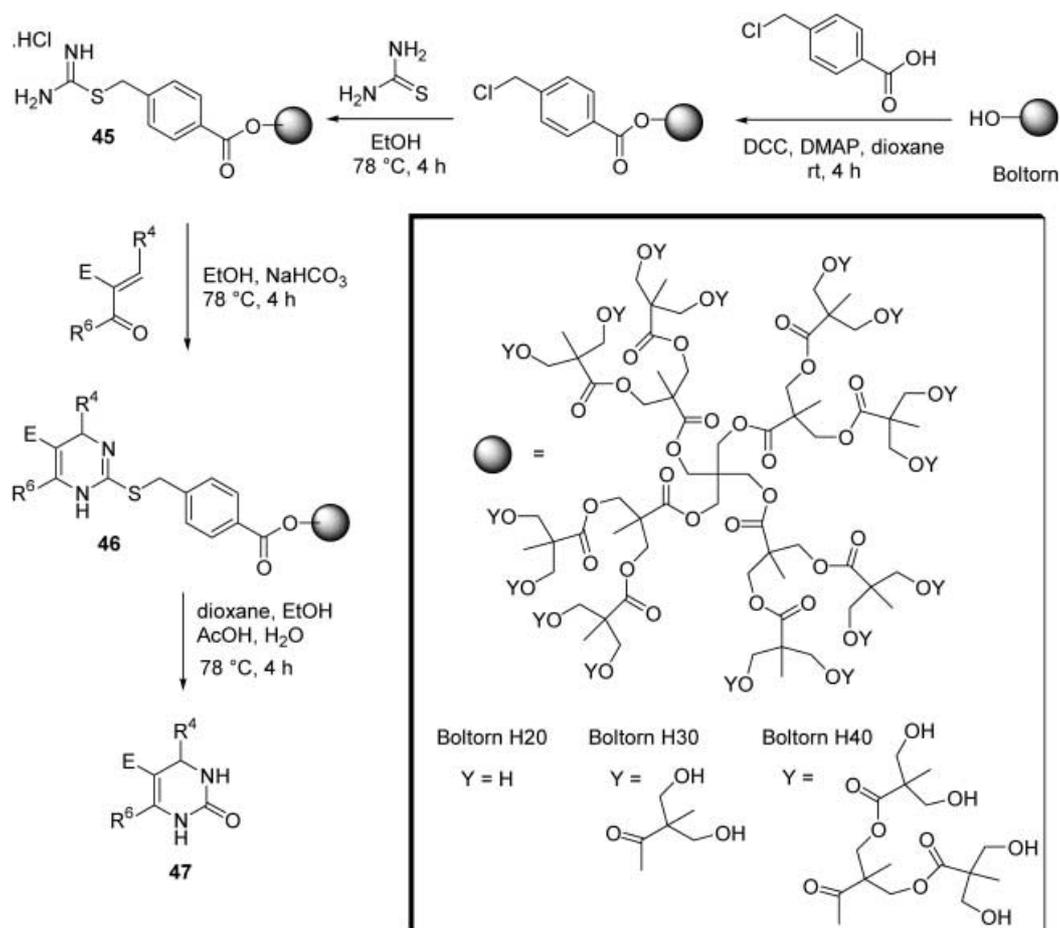
**Scheme 14.** Soluble polymer-assisted Biginelli condensation using hyperbranched star polymers [45].
