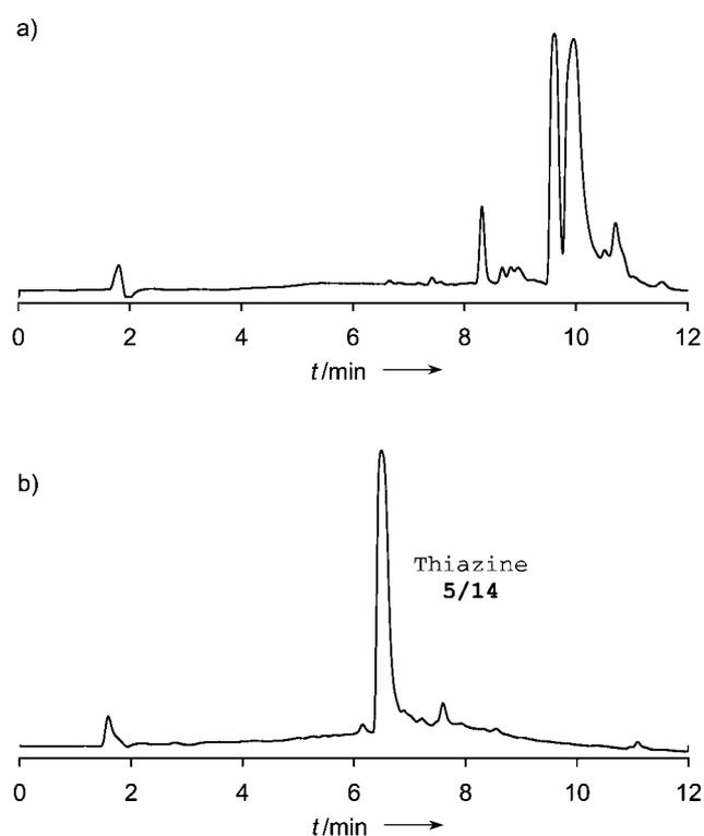
**Figure 2.** HPLC monitoring of thiazine synthesis. a) substances not bound to polymer-bound sulfonic acid in the selective sequestration step; b) final product **5/14**.
