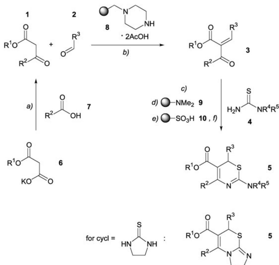
**Scheme 4.** a) (i) 1 equiv CDI, 1 equiv **7**, THF, RT, 3 h; (ii) 1 equiv **6**, 1.2 equiv MgCl<sub>2</sub>, MeCN, RT, 3 h; then add (i) to (ii), RT, 14 h; b) 1 equiv β-ketoester, 1.1 equiv aldehyde, 10 mol-% **8**, chlorobenzene, 115 °C, 5 h; c) 2.2 equiv **5**, 3 equiv 4 M HCl in dioxane, abs. ethanol, 80 °C, 8 h; d) 6 equiv **9**; e) 1.5 equiv **10**; f) wash step, then MeOH/TEA 3:1. CDI = *N,N'*-carbonyl diimidazole, TEA = triethylamine.
