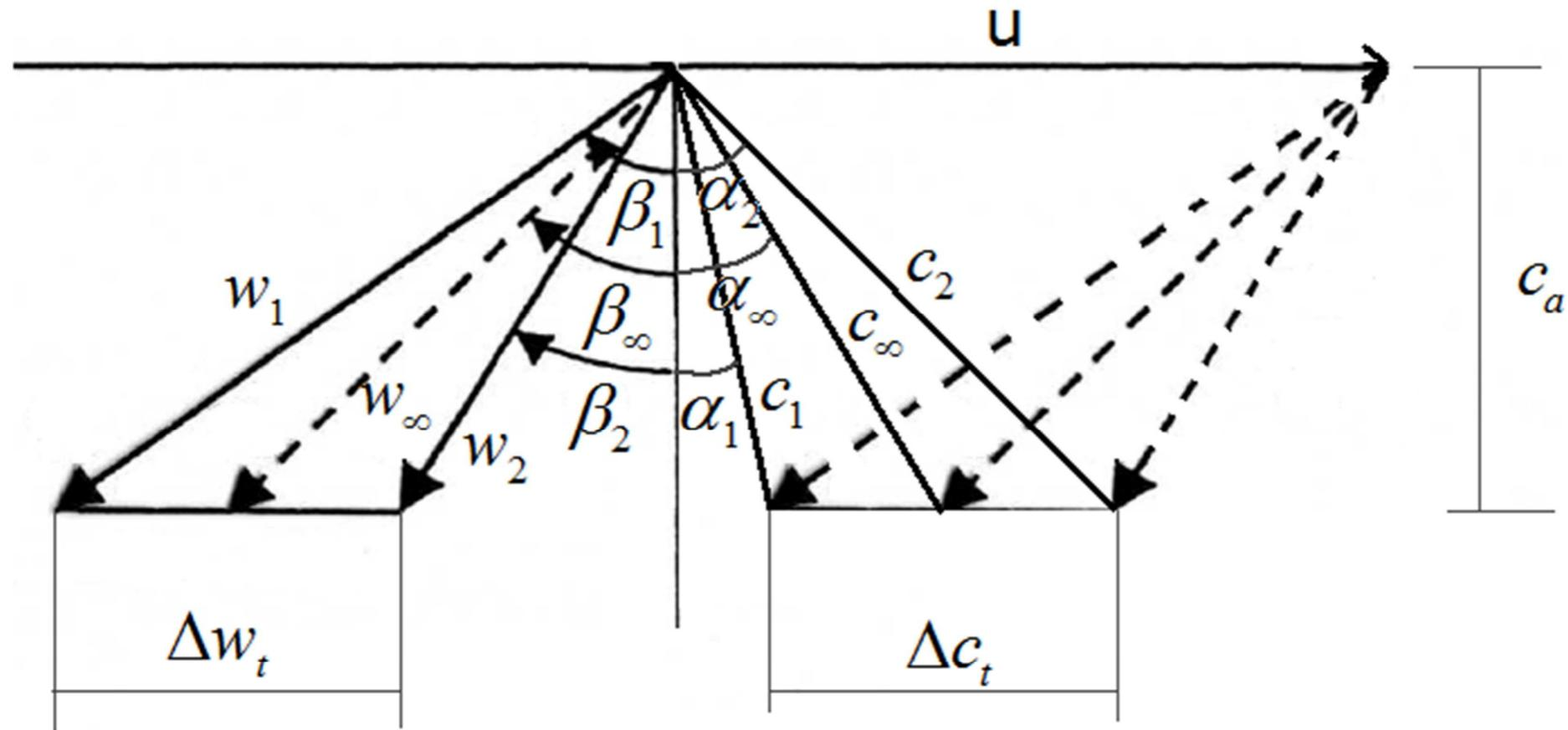
$$\Delta c_t = c_{2t} - c_{1t} = w_{1t} - w_{2t} = |\Delta w_t|$$
