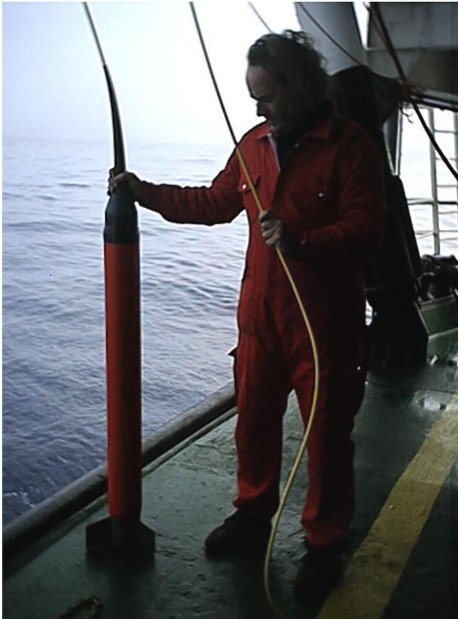
Instruments to measure the earth magnetic field in the ocean:
