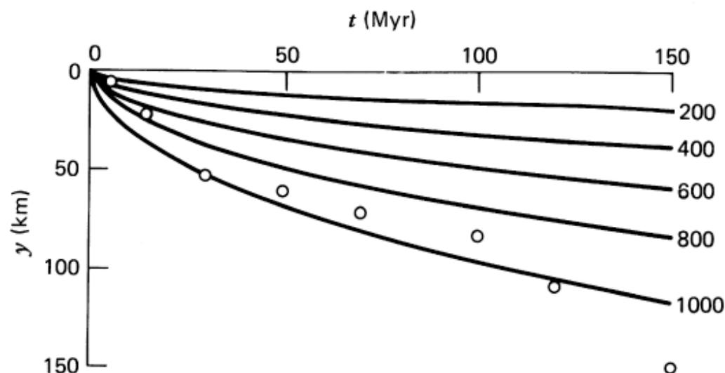
**Figure 4-24** The solid lines are isotherms,  $T - T_s$  ( $^{\circ}\text{K}$ ), in the oceanic lithosphere from Equation (4-125). The data points are the thicknesses of the oceanic lithosphere in the Pacific determined from studies of Rayleigh wave dispersion data. (From A. R. Leeds, L. Knopoff, and E. G. Kausel, Variations of upper mantle structure under the Pacific Ocean, *Science*, **186**, 141–143, 1974.)
