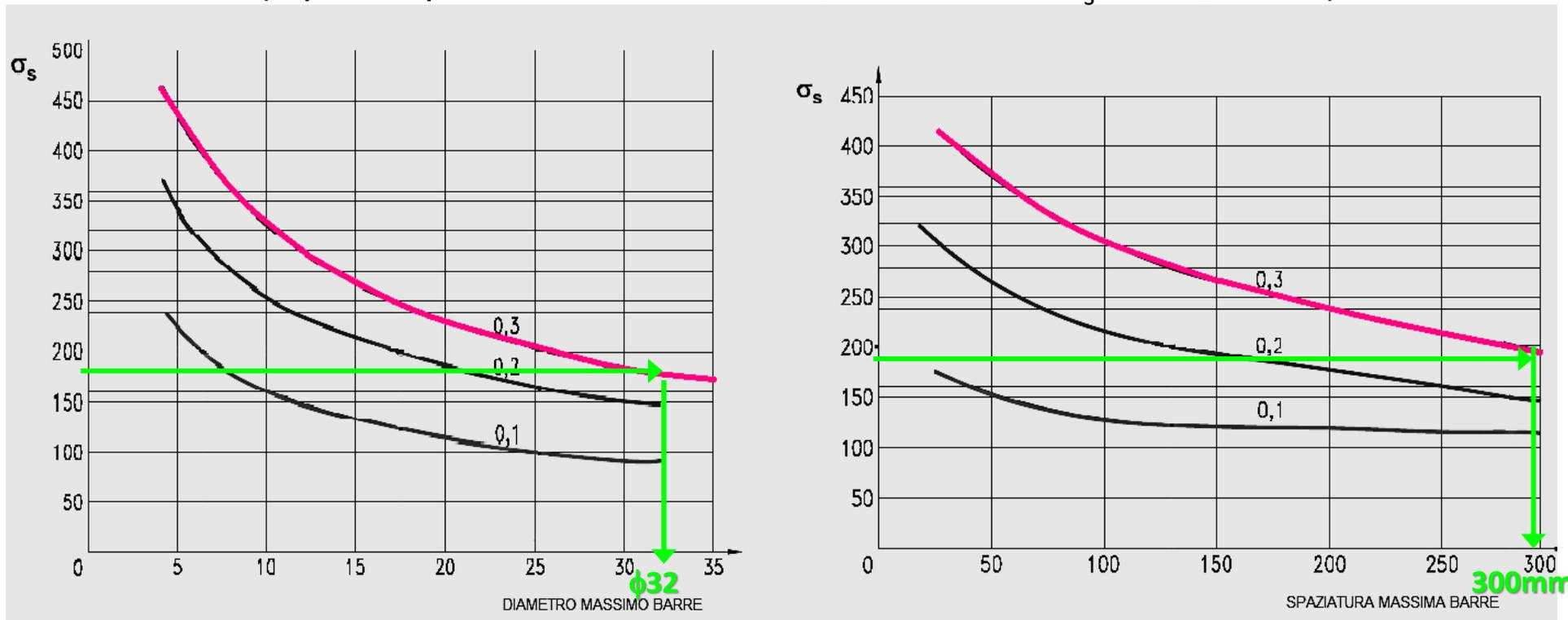
$\phi 14 < \phi 32$  e  $40 \text{ mm} < 300 \text{ mm}$  ✓ VERIFICATO
