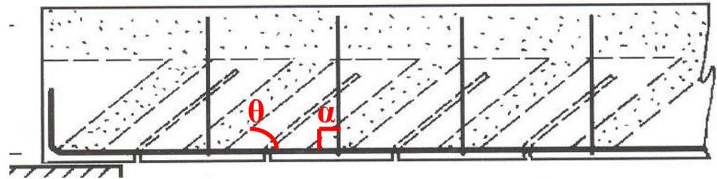
$$\Rightarrow V_{Rsd} = \frac{A_{sw}}{s} z f_{yd} ctg \vartheta$$
