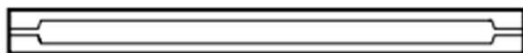
Figure 6: Thermo Scientific liner for TRACE 1300/1310 and Agilent Split/Splitless inlet, Double Taper 4 x 78.5 mm internal dimension (P/N 453A1355)
