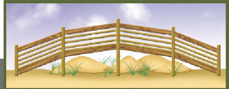
(B) Pier-supported with ramps
