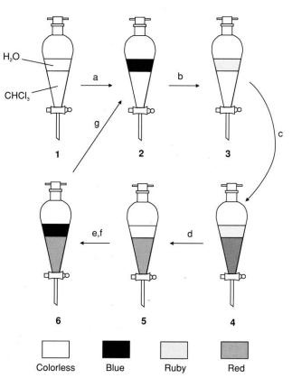
Effect of various operations on the appearance of the separatory funnel. In those operations where the separatory funnel is shaken, it is implicit that the layers are then allowed to separate. (a) Add A<sup>-</sup>; (b) Add 1 M HCl and stir aqueous layer; (c) Shake briefly; (d) Shake vigorously; (e) Add 1 M NaOH; (f) Shake gently; (g) Shake vigorously. This sequence of reactions is also shown in a color photograph on the cover of this issue.
