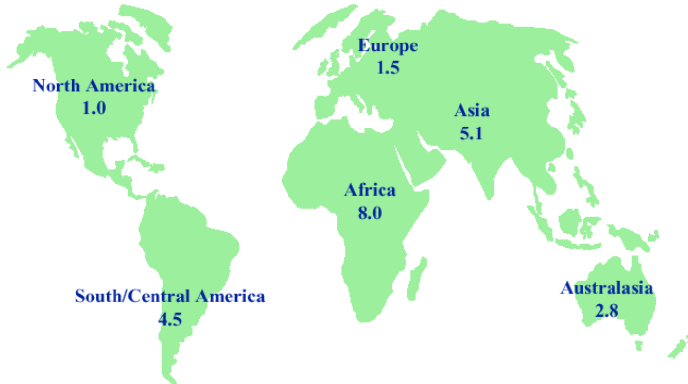
Figure 7.4.2 Accident locations - fatal accidents per million commercial ATMs
