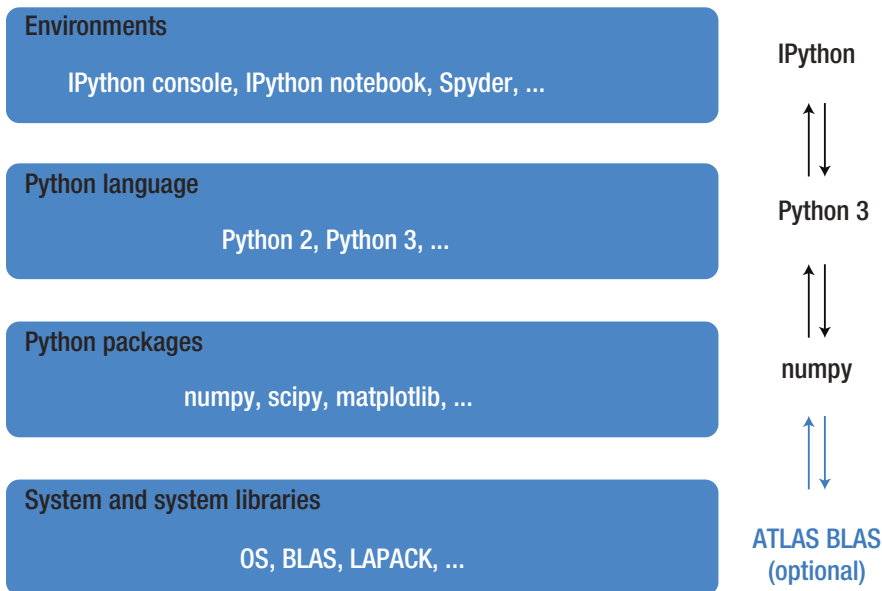
Figure 1-2. An overview of the components and layers in the scientific computing environment for Python, from a user's perspective, from top to bottom. Users typically only interact with the top three layers, but the bottom layer constitutes a very important part of the software stack. An example of specific software components from each layer in the stack is shown in the right part of the figure
