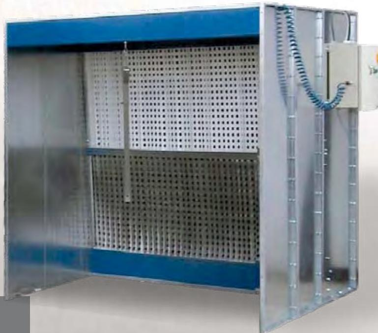
The **CBV** series spray booths are designed for paint, solvent, enamel, adhesive vapour extraction from works of small parts (glasses, helmet, miniatures/model-making). The spray booths are made of modular bended galvanized steel panels and are designed to convey all emissions toward the suction wall equipped with corrugated cardboard pre-filter ANDREAE® and a paint stop filter. An integral fan with reversed blades is set up allowing an optimal extraction.
