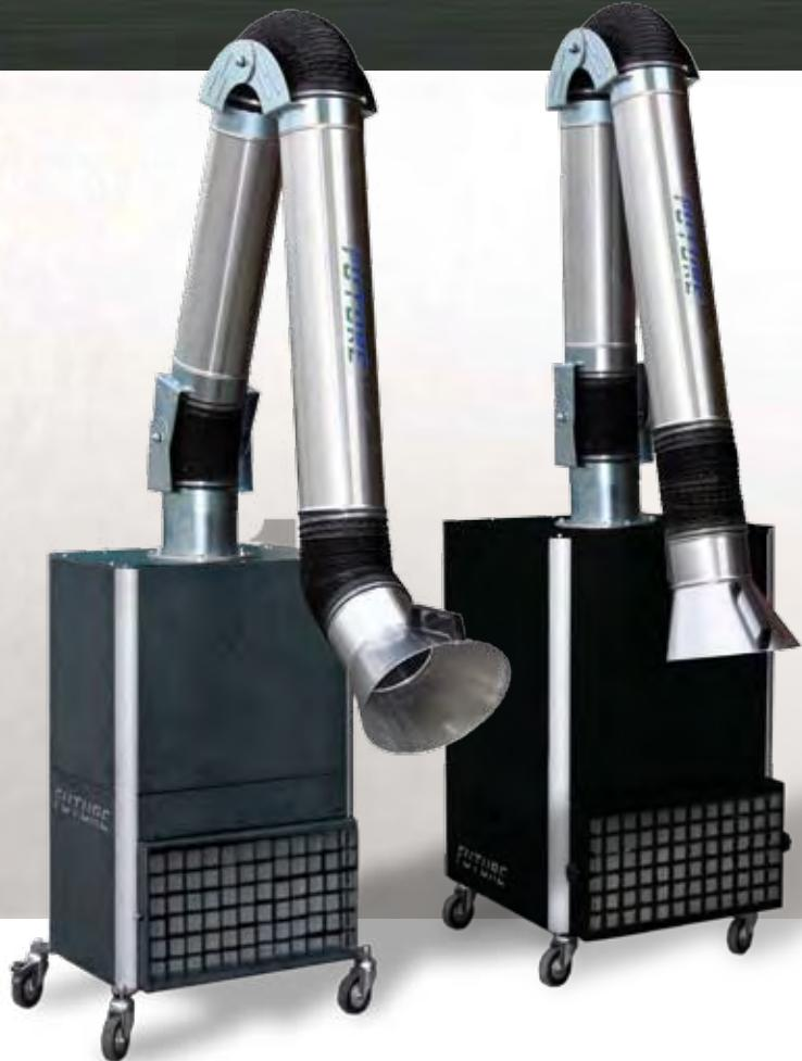
The mobile mechanical extractors, model AIR 2008 / AIR 2008 HT, have been designed for aspiration and filtration of fumes generated from the most common welding fumes GMAW – Gas Metal Arc Welding with CO<sub>2</sub>, SMAW – Shielded Metal with low hydrogen / rutile electrodes. The system is equipped with a diameter 200mm extraction arm, available in 3m length.
