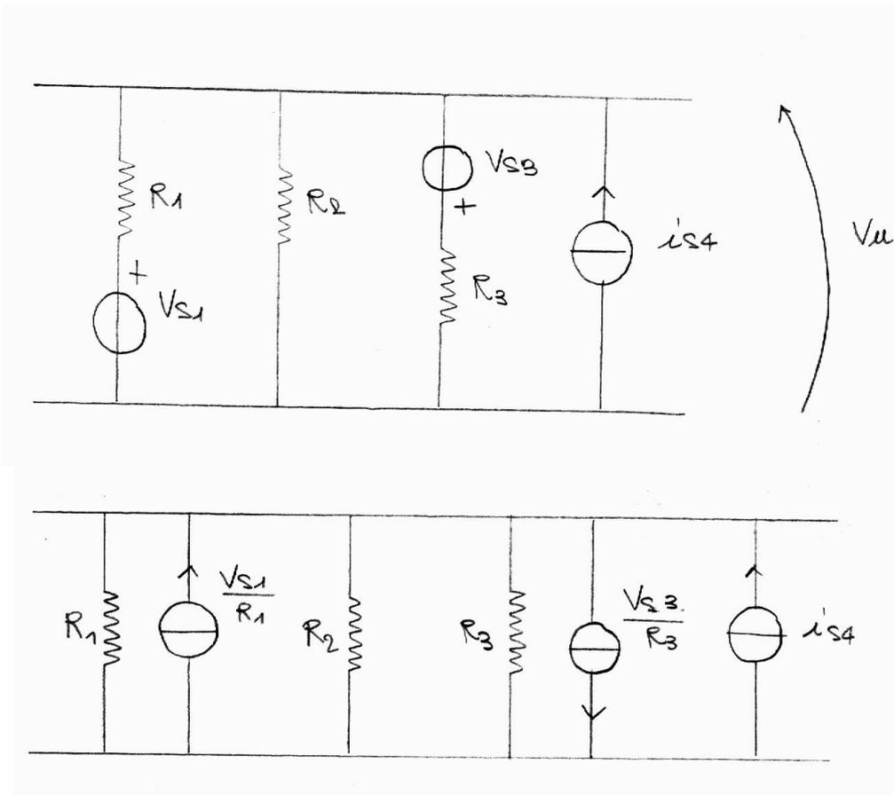
$$v_u = \frac{\frac{v_{s1}}{R_1} - \frac{v_{s3}}{R_3} + i_{s4}}{\frac{1}{R_1} + \frac{1}{R_2} + \frac{1}{R_3}}$$
