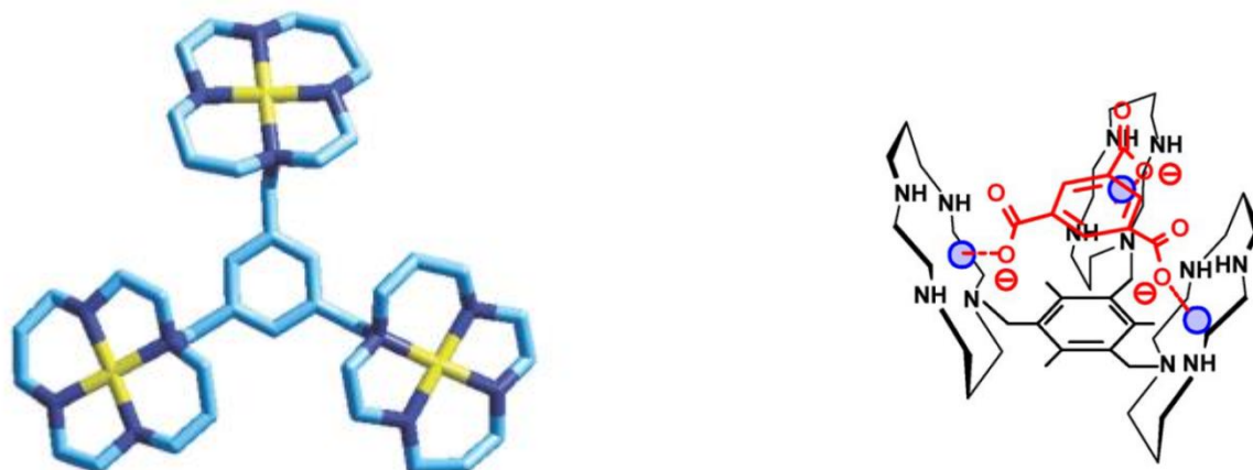
Fig. 25 The crystal structure of the complex salt [\text{Ni}_3(\mathbf{7a})](\text{ClO}_4)_6 \cdot \text{H}_2\text{O} . 58 Non-coordinating \text{ClO}_4^- ions and water molecule have been omitted for clarity, as well as hydrogen atoms. Each low-spin \text{Ni}^{\text{II}} centre shows a square coordination geometry.
