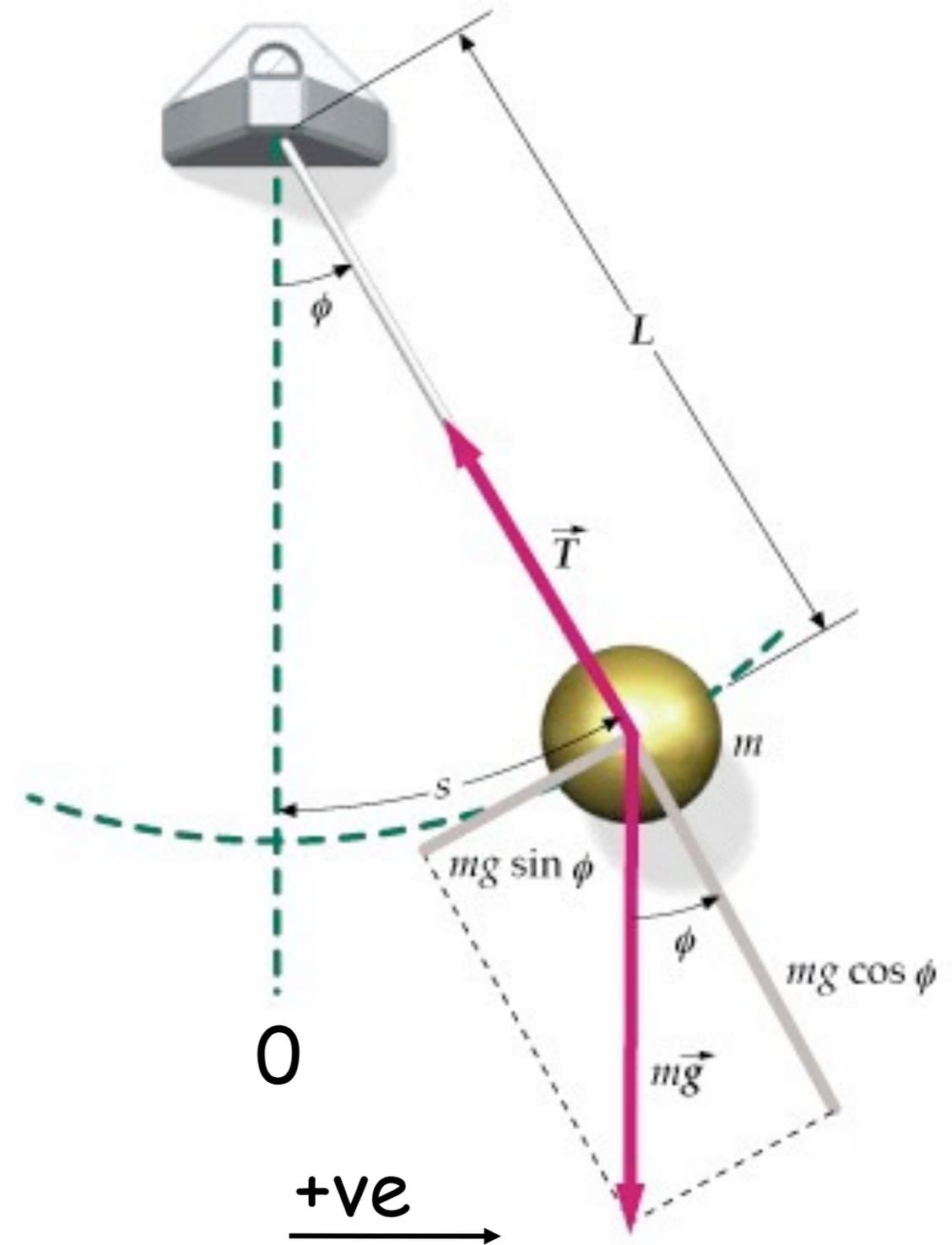
Per  $\frac{\phi(\text{rads})}{2\pi} = \frac{s}{2\pi L}$
