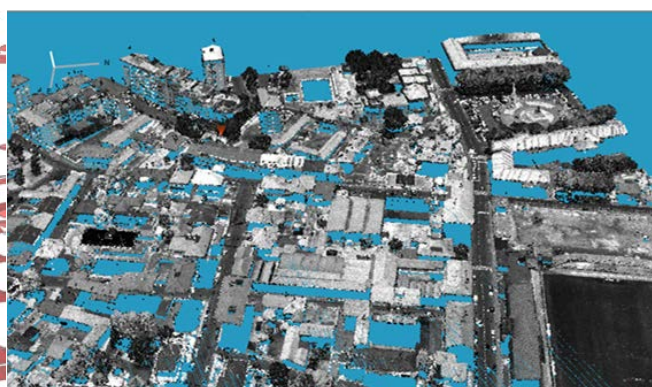
3D city model based on the LiDAR data, Turin
