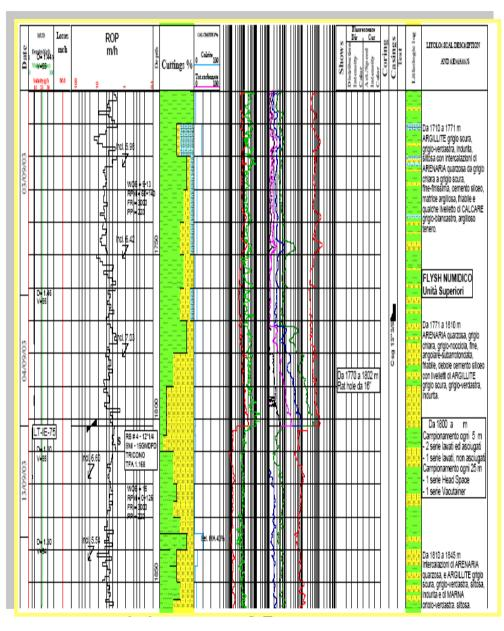
The Master Log (or Mud Log) is a document showing (in the form of a log) the variation of drilling parameters and while drilling information which are essential to the geological and petrophysical interpretation of well data (well logs included):
