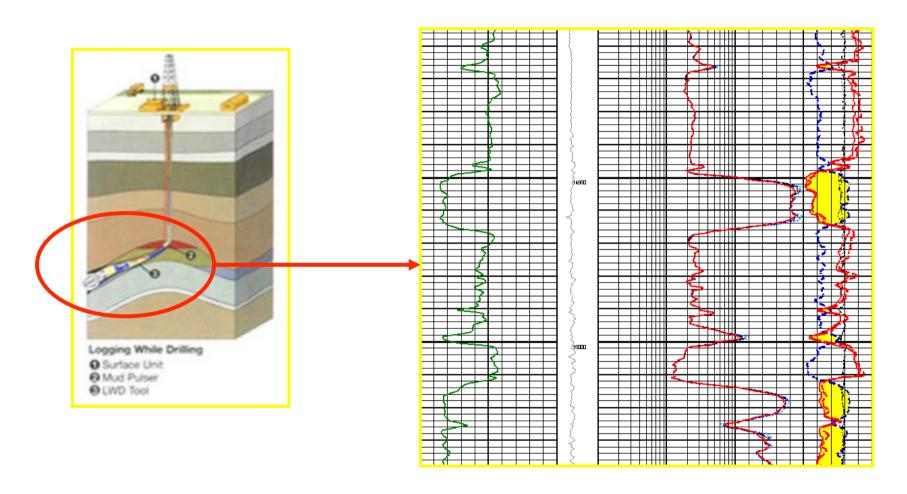
Modern Logging While Drilling technologies allow the acquisition of high quality logging curves (both in Real Time and Memory modes) for Real Time &/or Near Real Time Formation Evaluation and Geosteering.
