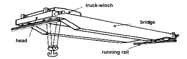
The bridge crane is a lifting construction that is subject to specific regulations that periodic verification. There are bridge cranes for loads ranging from tens kN to hundreds of kN (tens of tons).
