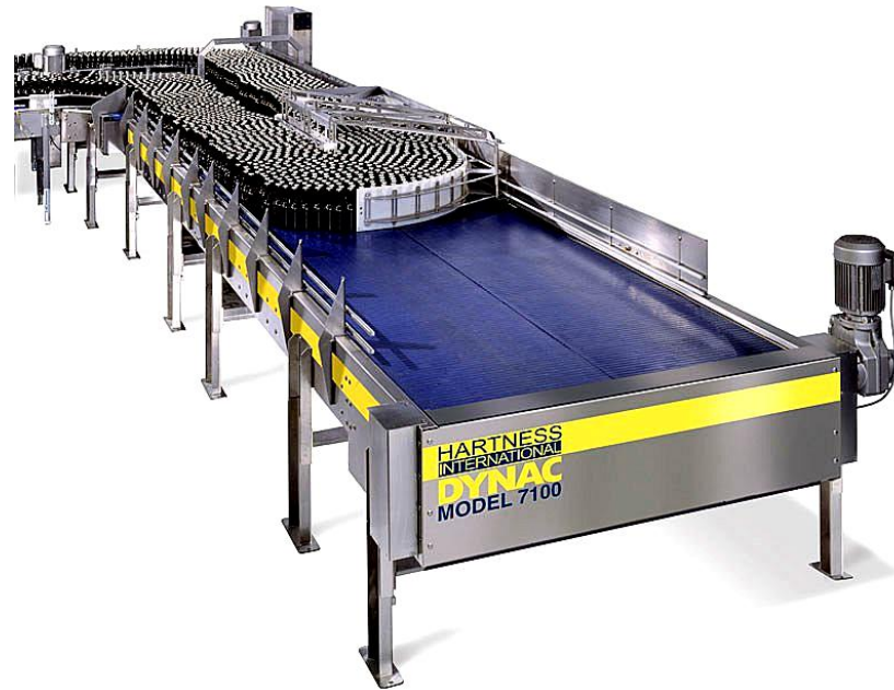
Belt conveyor to accumulation
