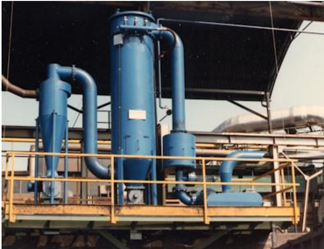
Pneumatic conveying for foundry sands
