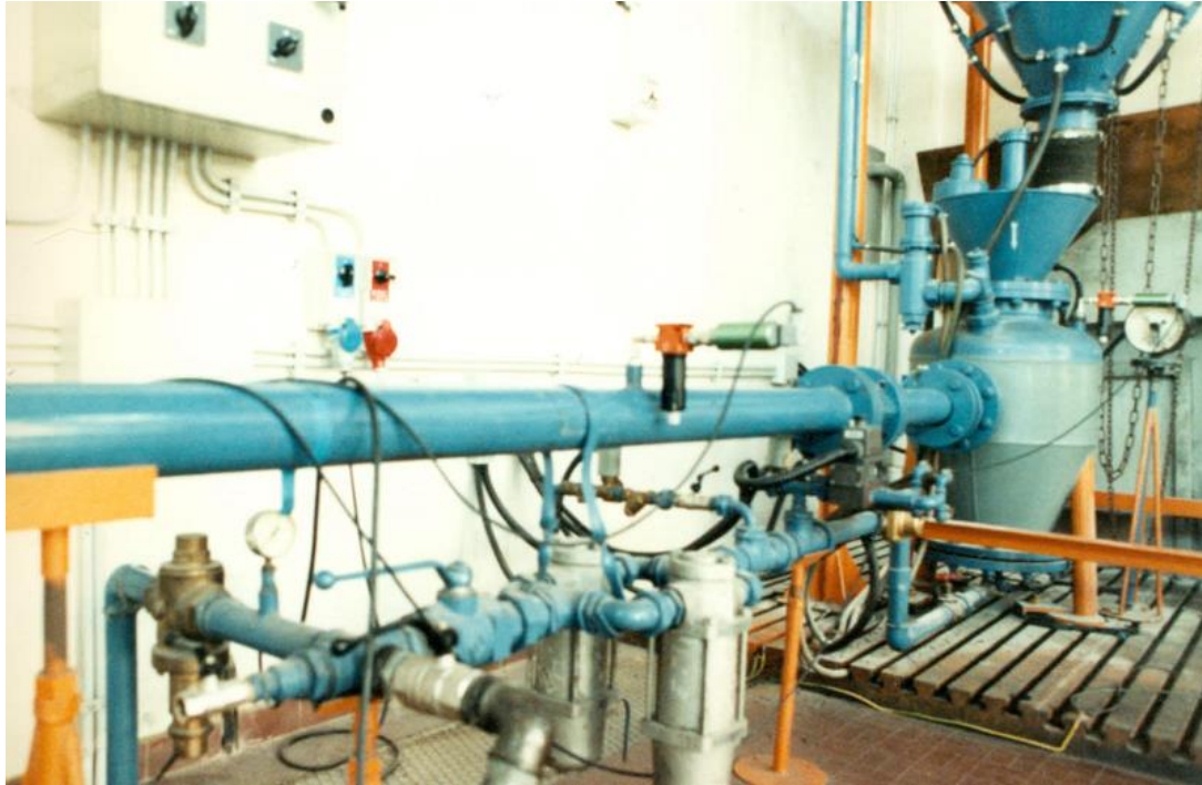
Pneumatic conveyor to push Propeller with the pipe of departure and a part of the supply circuit
