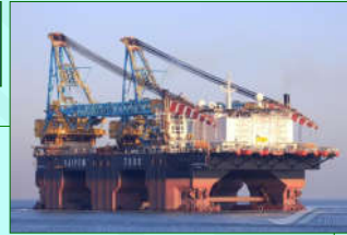
Crane vessel " Saipem 7000 " (Italian, but Bahamas Flag) Crew: 400 7,000t each crane. Speed: 32 knots The biggest in the world, of its type.
