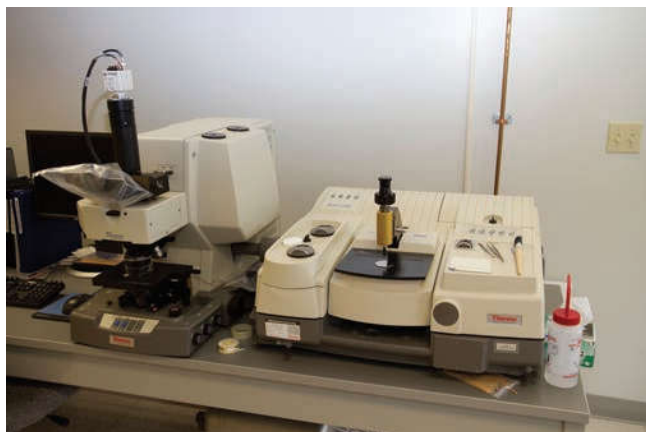
Fig. 4.11 Fourier transform (FT) IR spectrometer in a forensic crime laboratory.
