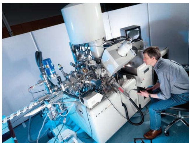
Fig. 4.35 An X-ray photoelectron spectrometer (XPS) being used to analyse the surface of a material.
