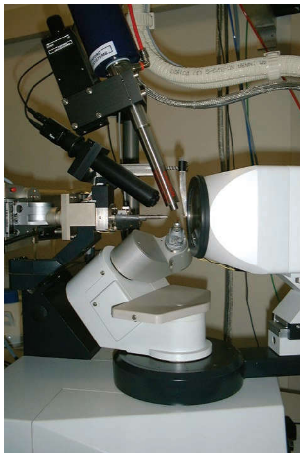
Fig. 4.30 A Kappa-CCD diffractometer equipped with a nitrogen gas, low-temperature cryostat (upper, centre in the photograph). The X-ray source and the detector are on the left- and right-hand sides of the photograph, respectively. The crystal is mounted on the goniometer head (centre). The black 'tube' shown at the upper left is a microscope.
