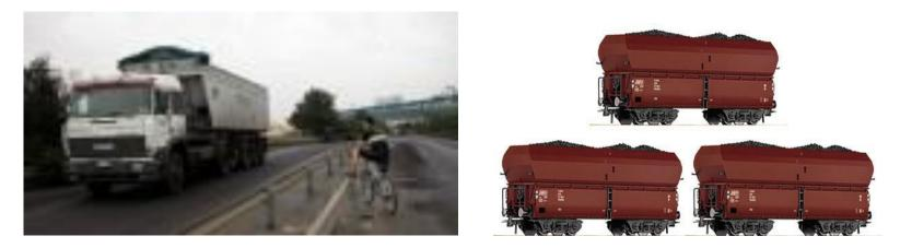
Both trucks that the wagons are specially shaped to easily download the solid fuel by lift and tilt of the body itself by the hydraulic pistons or opening of the side doors of the body.
