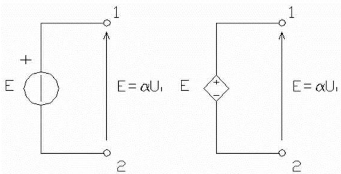
VCVS = Voltage Controlled Voltage Source
