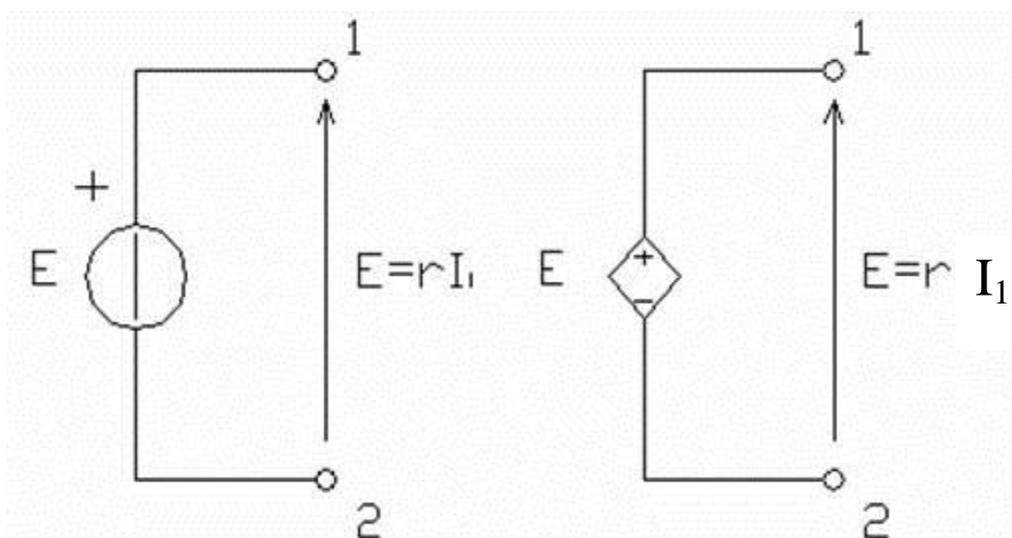
CCVS = Current Controlled Voltage Source
