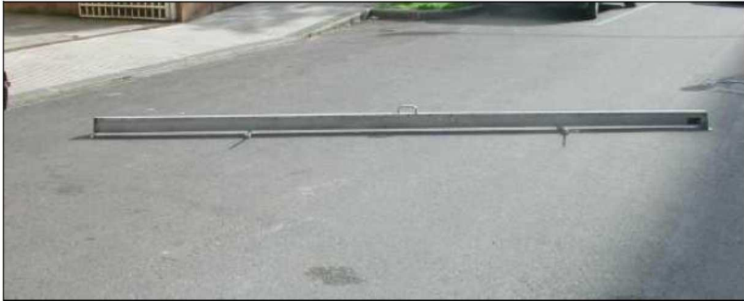
Profile Measurement: Dipstick Profiler
