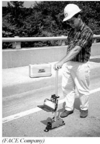
Profile Measurement: Dipstick Profiler
