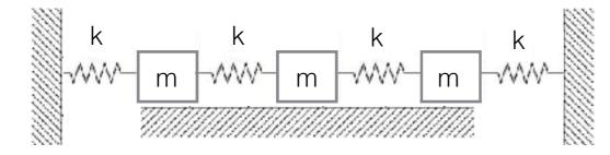
$$\begin{bmatrix} D(\omega) \end{bmatrix} = \begin{bmatrix} 2 - \omega^2 & -1 & 0 \\ -1 & 2 - \omega^2 & -1 \\ 0 & -1 & 2 - \omega^2 \end{bmatrix}$$
