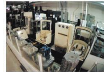
Robotic Modular Machining Cell
