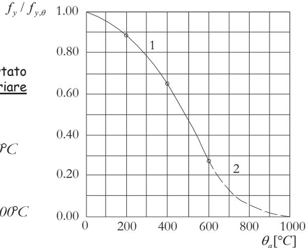
$$f_{y,\theta} = f_y \left[ 1 + \frac{\theta_a}{767 \ln(\theta_a/1750)} \right] \quad 0^\circ\text{C} \leq \theta_a \leq 600^\circ\text{C}$$
