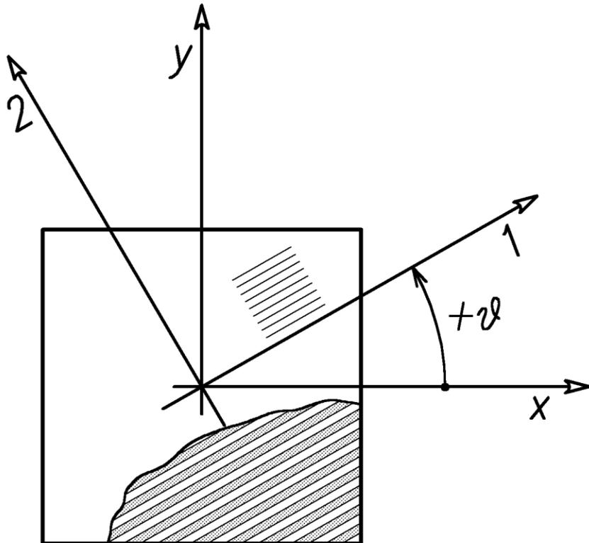
$$\begin{Bmatrix} \sigma_1 \\ \sigma_2 \\ \tau_{12} \end{Bmatrix} = \underline{\underline{T}}(\theta) \begin{Bmatrix} \sigma_x \\ \sigma_y \\ \tau_{xy} \end{Bmatrix}$$
