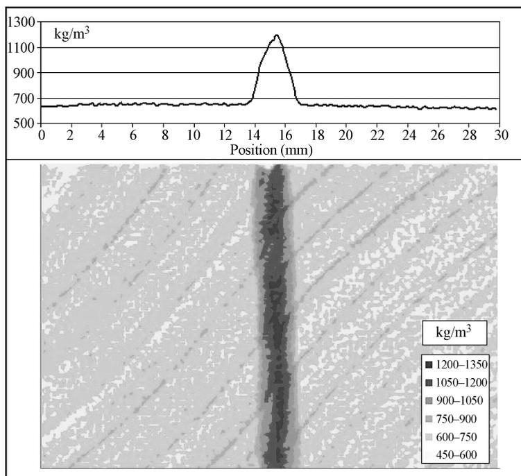
**Figure 3.** X-ray microdensitometry map of friction welded hydrothermally treated birch wood. Upper microdensitometry graph expresses density in  $\text{kg/m}^3$  of the wood as a function of the sample weld interface position in mm. The bottom panel is the color intensity microdensitometry map expressing increasing density in  $\text{kg/m}^3$  by progressive darkening. Scale of sample weld interface position is the same for the two panels.
