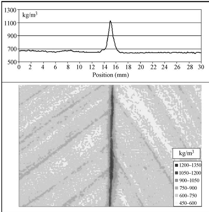
**Figure 4.** X-ray microdensitometry map of friction welded birch wood after final dry heat cure treatment. Upper microdensitometry graph expresses density in  $\text{kg/m}^3$  of the wood as a function of the sample weld interface position in mm. The bottom panel is the color intensity microdensitometry map expressing increasing density in  $\text{kg/m}^3$  by progressive darkening. Scale of sample weld interface position is the same for the two panels.
