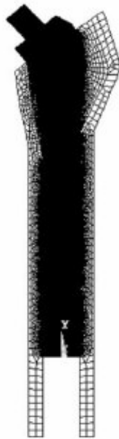
Figure 4. The finite element mesh for the endoprosthesis.
