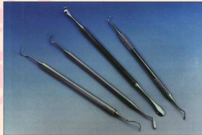
Biomateriali These dental instruments require alloys that have good corrosion resistance, machinability, and edge retention.
