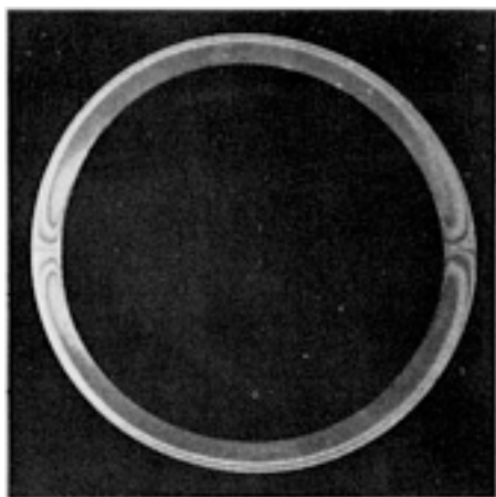
Fig. 3 Alloy 3003-F tube, extruded through a two-port bridge die. The bands of fine precipitate
