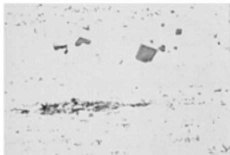
Fig. 4 Alloy 3003-F sheet, hot rolled. Longitudinal section shows stringer of oxide from an inclusion in the cast ingot and particles of phases that contain manganese, both primary (large, angular) and eutectic (small). As-polished. 500×
