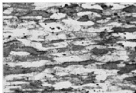
Fig. 5 Alloy 3003-O sheet, annealed. Longitudinal section shows recrystallized grains. Grain elongation indicates rolling direction, but not the crystallographic orientation within each grain. Polarized light. Barker's reagent. 100×
