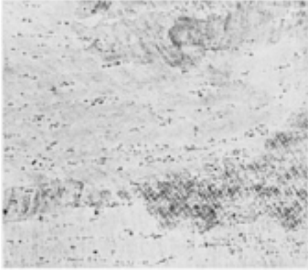
Fig. 54 Same alloy and heat treatment as Fig. 53 , but showing no recrystallization of the worked structure. Note the large amount of slip (light parallel lines) that has occurred on two sets of slip planes. Keller's reagent. 100×
