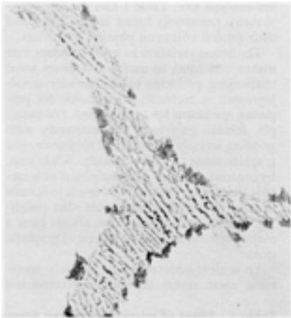
Fig. 13 ASTM A128 grade A alloy, cast and deliberately overheated to 1205 °C (2200 °F) for 1 h, then water quenched. Photomicrograph illustrates a triple point in the austenite grain structure, with detail of the eutectic pattern of incipient fusion associated with the carbide due to excessive solutionizing temperature. Cyclic etch (see Table 1 for composition and method). 500×
