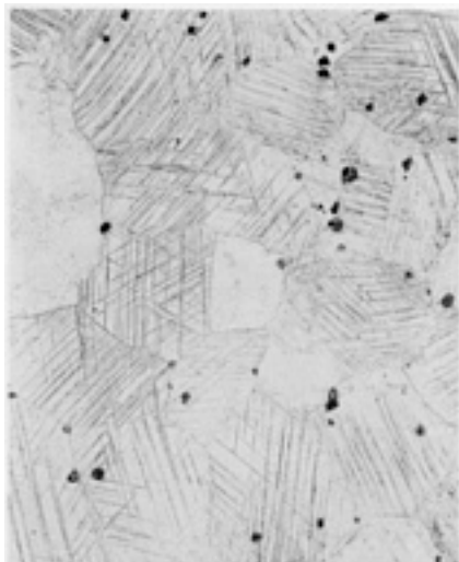
Fig. 6 ASTM A128 alloy, cast and heat treated at 1065 °C (1950 °F), water quenched, machined into tensile specimen, and tested. Austenite grains show different amounts of twinning, depending on individual grain orientation. Etchant: Same as Fig. 5 . 100×
