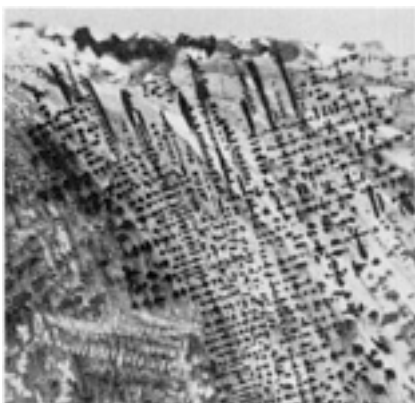
Fig. 3 Same material as Fig. 1 , static cast. Grains from the chilled bottom grew through the dendrite "skeletons," producing a mixed grain structure, Etchant 10, Table 3 . 3x
