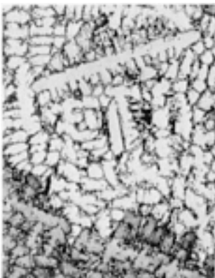
Fig. 7 Same material as Fig. 6 , with primary dendrites of \alpha phase darkened. Lead appears as small spheroids. Etchant 1, Table 3 . 50×. (J. Dibee)
