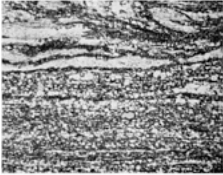
Fig. 18 HM31A-T5 extrusion. Longitudinal view of banded hot-worked structure. Small, recrystallized grains; dark Mg_4Th grain-boundary precipitate; light islands are solid solution rich in thorium and so more resistant to hot working; gray particle is manganese. Etchant 5, Table 1 . 500×
