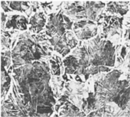
Fig. 15 Overheated ASTM A515, Grade 70, steel plate, 38 mm (1.5 in.) thick. Normalized by austenitizing at 1125 °C (2060 °F) for 1.5 h and air cooling. Note ferrite at prior austenite grain boundaries and within grains. 1% nital. 100×
