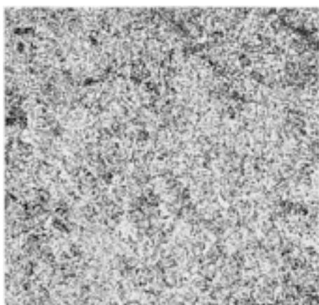
Fig. 23 ASTM A533, Grade B, steel plate, 300 mm (12 in.) thick. Austenitized at 915 °C (1675 °F) for 12 h, water quenched, re-austenitized at 855 °C (1575 °F) for 12 h, water quenched, tempered at 665 °C (1225 °F) for 12 h, air cooled, and stress relieved twice: 40 h at 605 °C (1125 °F) and 42 h at 550 °C (1025 °F). See also Fig. 24 . Saturated picral. 250×
