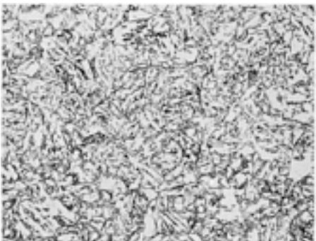
Fig. 27 Same steel and heat treatment as for Fig. 23 , but specimen was taken from center of plate. Structure is largely tempered bainite; some proeutectoid ferrite (more equiaxed light gray constituent) is evident. Saturated picral. 250×
