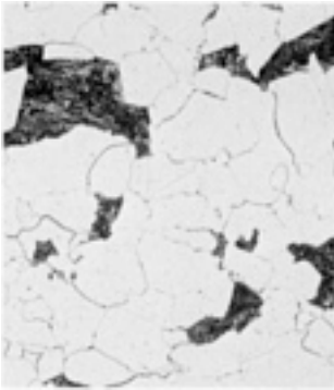
Fig. 51 Same as Fig. 50 , but 50-mm (2-in.) thick as-rolled plate. Structure consists of polygonal ferrite-pearlite. Note effect of gage dimension on grain size (compare with Fig. 50 ). Nital plus picral. 500×
