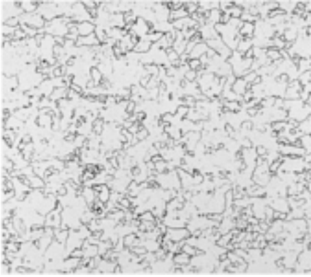
Fig. 41 ASTM A562 steel plate, 25 mm (1 in.) thick. Normalized by austenitizing at 900 °C (1650 °F) for 1 h and cooling in air. The microstructure consists largely of ferrite, with small particles of titanium carbide. 1% nital. 100×
