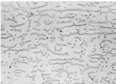
**Fig. 28** Same sand cast alloy and section thickness as [Fig. 26](#), but solution treated 1 h at 1120 °C (2050 °F) and water quenched. Structure: pools of ferrite (outlined) in austenite; dendritic pattern has been altered. Glyceregia. 100×
