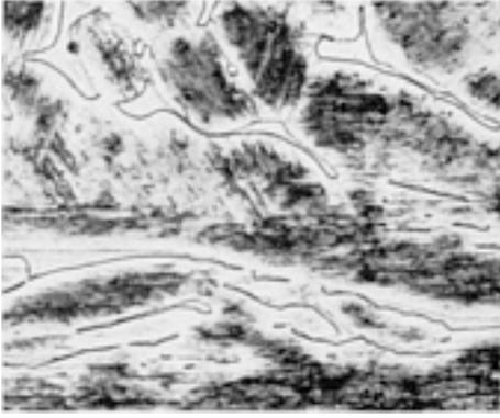
**Fig. 14** CB-7Cu-1 alloy, as-cast. The structure consists of elongated pools of ferrite (light gray constituent) in a matrix of martensite, which varies in carbon content (as indicated by the response to etching). See also [Fig. 15](#). Vilella's reagent. 500×
