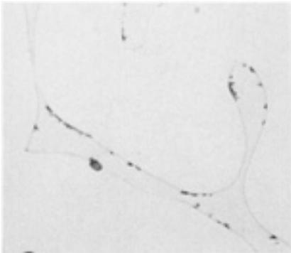
**Fig. 34** Same alloy and processing as [Fig. 33](#). Higher magnification of austenite, ferrite and carbide precipitates at interface. Kalling's reagent. 1000×
