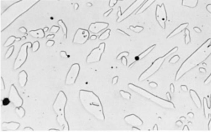
**Fig. 17** Same alloy as for [Fig. 16](#), but solution treated at 1065 °C (1950 °F) for 1 h and water quenched. Shows effect of homogenization. Electrolytic: 10% CrO<sub>3</sub> at 6 V for 5 to 60 s. 500×
