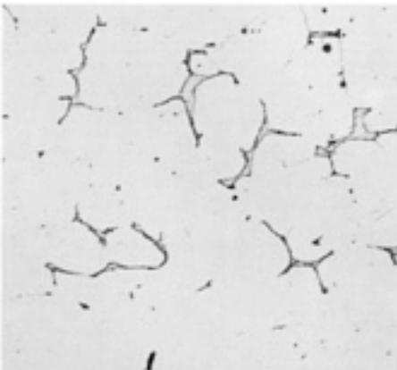
**Fig. 22** CF-3 alloy, 150-mm (6-in.) thick section, as-cast, showing dispersed islands of ferrite (5% by volume) and grain-boundary carbide particles in an austenite matrix. See also [Fig. 23](#). HCl, HNO<sub>3</sub>, acetic acid. 100 $\times$
