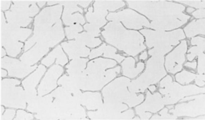
**Fig. 30** CF-8 alloy, 150-mm (6-in.) thick section, as-cast. Similar in ferrite distribution to [Fig. 29](#). Note that chromium carbide particles have precipitated at the ferrite-austenite boundaries. Matrix is austenite. See also [Fig. 31](#). Electrolytic: KOH. 200×
