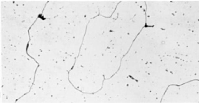
**Fig. 38** CF-20 alloy, a 25-mm (1-in.) bar, as-cast. The structure consists of fine particles of carbide dispersed in a matrix of austenite with precipitated carbide particles at grain boundaries. Oxalic acid. 100×
