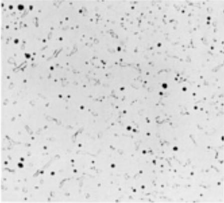
**Fig. 36** Same alloy and bar size as for [Fig. 35](#), but solution treated at 1120 °C (2050 °F) and water quenched. The precipitated carbide particles have dissolved, and the ferrite islands have re-formed. Selenide particles (black) were relatively unaffected by the solution treatment. Electrolytic: oxalic acid. 100×
