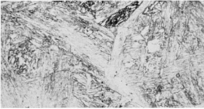
**Fig. 4** CA-6NM alloy, 75-mm (3-in.) thick section, heated to 1050 °C (1925 °F) and held 3 h, air cooled, tempered 1 h at 605 °C (1125 °F). Ferrite-free tempered martensite, but coarser than in [Fig. 3](#). See also [Fig. 5](#). Vilella's reagent. 500×
