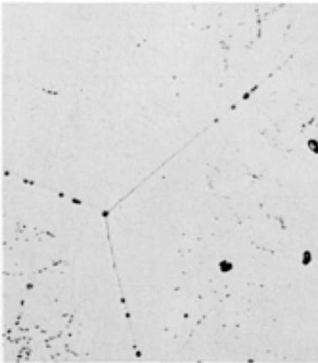
**Fig. 46** Same alloy and section thickness as for [Fig. 45](#), but solution treated at 1120 °C (2050 °F) for 1 h and water quenched. Small discrete chromium carbide particles at grain boundaries of the etch-pitted austenite matrix. Electrolytic: oxalic acid. 500×
