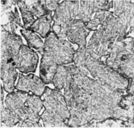
**Fig. 8** Same alloy, section thickness, and condition as [Fig. 7](#), but a different casting, etchant, and magnification. Structure consists of islands of ferrite and grain-boundary carbide (dark) in martensite matrix. See [Fig. 9](#). Ferric chloride. 100×
