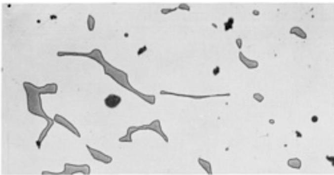
**Fig. 37** CF-16F alloy, solution treated at 1120 °C (2050 °F) and water quenched. The structure consists of selenide particles (dark spots) and islands of ferrite in a matrix of austenite. Electrolytic: 10N KOH. 500×
