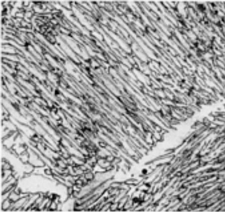
**Fig. 24** CF-3M alloy, as-cast. Specimen taken from a 25-mm (1-in.) thick section. Structure consists of a complex network of elongated ferrite in a matrix of austenite. Ferrite content is estimated at 22%. HCl, HNO<sub>3</sub>, acetic acid. 100×
