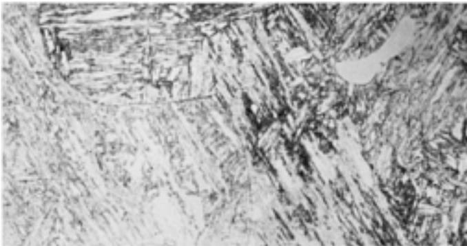
**Fig. 5** Same alloy and heat treatment as for [Fig. 4](#), but a section 150-mm (6-in.) thick. Some ferrite (note pool in upper right corner) is present in the tempered martensite matrix. Vilella's reagent. 500×
