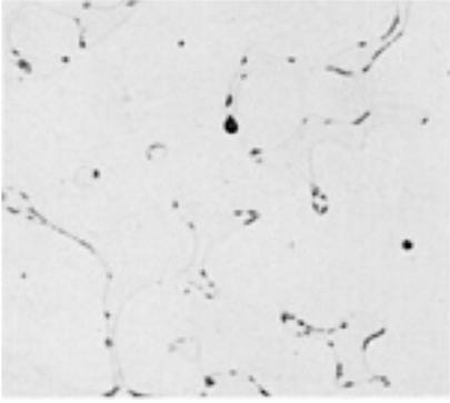
**Fig. 33** CF-8M alloy, solution treated 1 h at 1120 °C (2050 °F) and water quenched, sensitized 1 h at 650 °C (1200 °F) and air cooled. Structure is austenite, with ferrite and carbide precipitates along the austenite-ferrite interface. See also [Fig. 34](#). Glyceregia. 400×
