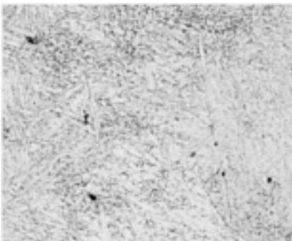
**Fig. 6** CA-15 alloy, normalized 4 h at 980 °C (1800 °F) and tempered 6 h at 705 °C (1300 °F). Structure consists of tempered martensite. Vilella's reagent. 400×
