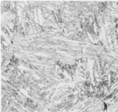
**Fig. 1** CA-6NM alloy, normalized 1 h at 1010 °C (1850 °F) and tempered 2 h at 650 °C (1200 °F). Structure consists of tempered martensite. Vilella's reagent. 400×
