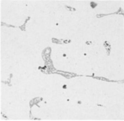
**Fig. 20** CF-3M alloy, solution treated 1 h at 1120 °C (2050 °F), water quenched and reheated 100 h at 760 °C (1400 °F). Structure is austenite matrix with some  $\sigma$ -phase present. See also [Fig. 21](#). Electrolytic: NaCN. 400 $\times$
