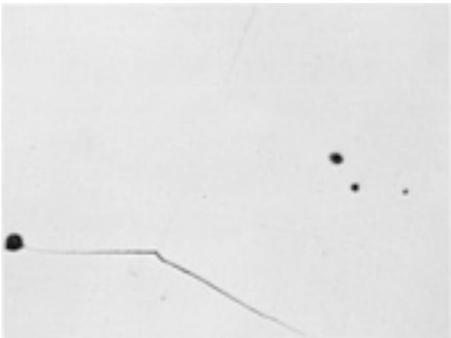
**Fig. 41** CN-7M alloy, 25-mm (1-in.) thick section, as-cast- Precipitated chromium carbide ( $M_{33}C_6$ ) at grain boundaries of the austenite matrix. Black dots are inclusions. See also [Fig. 42](#). Electrolytic: 10%  $CrO_3$ ; 6 V, 5 to 60 s. 500×
