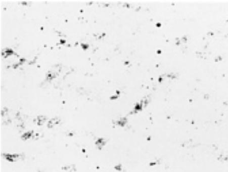
**Fig. 40** Same alloy and section thickness as for [Fig. 39](#), but solution treated at 1120 °C (2050 °F) for 1 h and water quenched. Most precipitated carbide particles have dissolved. Electrolytic: oxalic acid. 100×
