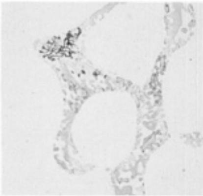
**Fig. 21** Same alloy and processing as [Fig. 20](#). Higher magnification of  $\sigma$ -phase in austenite. Electrolytic: NaCN. 1000 $\times$
