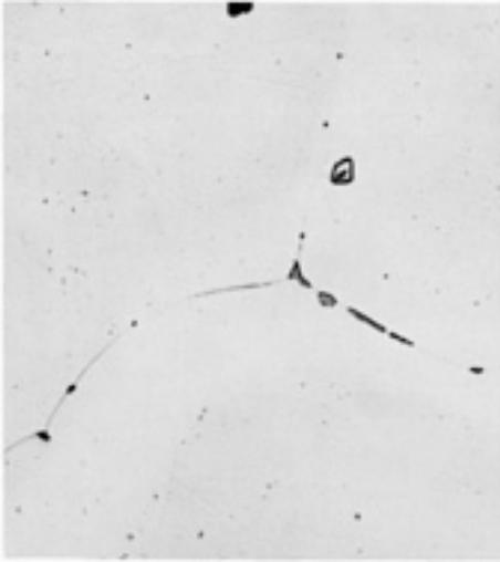
**Fig. 45** CN-7M alloy, 75-mm (3-in.) thick section, as-cast. The structure consists of  $M_{23}C_6$  carbides (predominantly, chromium carbide) precipitated at the grain boundaries of the austenite matrix. See also [Fig. 46](#). Electrolytic: oxalic acid. 500×
