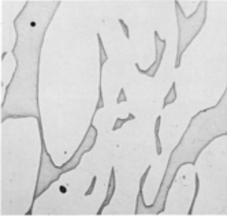
**Fig. 23** Same alloy and section thickness as for [Fig. 22](#), but solution treated at 1120 °C (2050 °F) and water quenched. Specimen was taken from center of section. Elongated pools of ferrite in an austenite matrix (light). Electrolytic: 10N KOH. 250×
