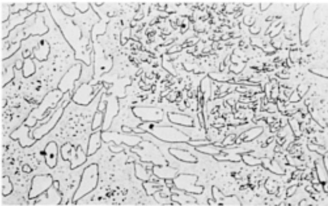
**Fig. 16** CD-4MCu alloy, as-cast. Structure: jagged pools and particles of austenite in ferrite. Black specks are nonmetallic inclusions. Electrolytic: 10% CrO<sub>3</sub> at 6 V for 5 to 60 s. 500×
