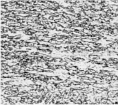
**Fig. 11** Same alloy, section thickness, and heat treatment as for [Fig. 11](#), but at a higher magnification to emphasize the traces of ferrite in the tempered martensite matrix. Hardness of casting, 223 HB. Vilella's reagent. 500×
