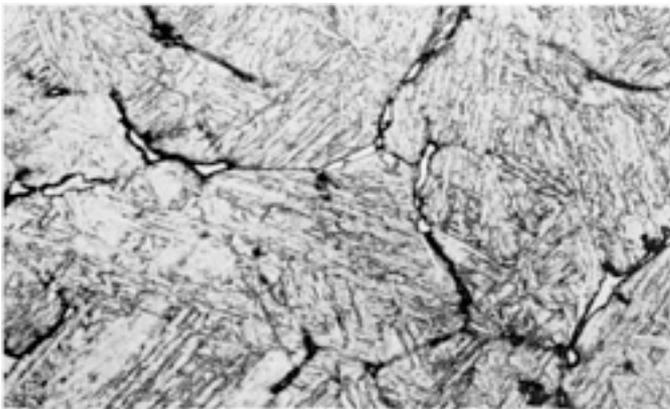
**Fig. 2** CA-6NM alloy, 75-mm (3-in.) thick section, as-cast. Cooling rate was very slow (casting was made in a sand mold). Precipitated chromium carbide particles (dark) and ferrite (white) are present at grain boundaries in a matrix of low-carbon martensite. See also [Fig. 3](#). Vilella's reagent. 200×
