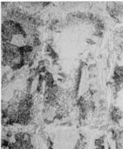
**Fig. 47** 440C stainless (Fe-17Cr-0.5Mo-1.0C), investment cast in a 5 mm (0.19 in.) section and annealed. Dendritic structure with interdendritic carbide network. See also [Fig. 48](#). Vilella's reagent. 500×
