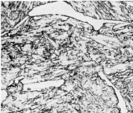
**Fig. 13** Same alloy, section thickness, and heat treatment as for [Fig. 12](#), but at a higher magnification to reveal dispersed ferrite particles and massive ferrite stringers in the tempered martensite matrix. Vilella's reagent. 500×
