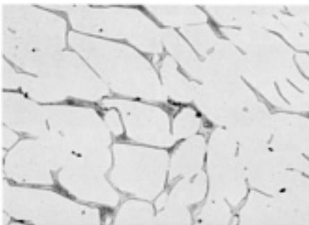
**Fig. 29** CF-8 alloy, 25-mm (1-in.) thick section, as-cast. The structure consists of a network of
