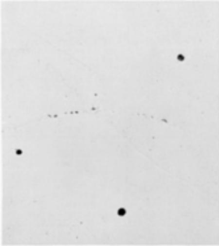
**Fig. 42** Same alloy and section thickness as for [Fig. 41](#), but solution treated 1 h at 1120 °C (2050 °F) and water quenched. Structure shows traces of carbide at grain boundaries of the austenite matrix; black dots are inclusions. Electrolytic: 10% CrO<sub>3</sub>; 6 V, 5 to 60 s. 500×
