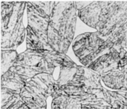
**Fig. 15** Same alloy as [Fig. 14](#), but austenitized at 1050 °C (1925 °F) for 1 h and aged at 495 °C (925 °F). The matrix, tempered martensite, still contains ferrite pools (light), but shows less variation in carbon content. Vilella's reagent. 500×
