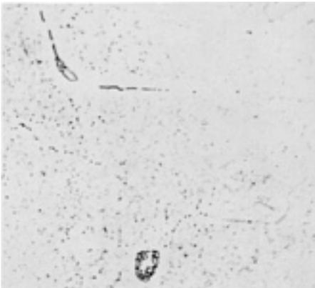
**Fig. 32** CF-8C alloy, solution treated at 1120 °C (2050 °F) for 1 h, water quenched, stabilized at 925 °C (1700 °F) for 1 h. Niobium carbide particles (black) precipitated during stabilization treatment at 925 °C (1700 °F). Remaining structure: ferrite in austenite matrix. Electrolytic: 10% CrO<sub>3</sub>; 6 V, 5 to 60 s. 500×
