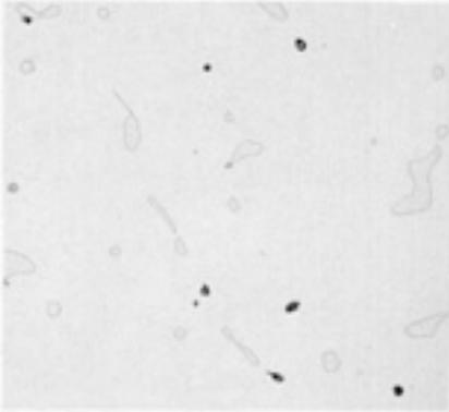
**Fig. 18** CF-3 alloy, solution treated 1 h at 1120 °C (2050 °F) and water quenched. Structure is austenite, with ferrite pools and inclusions. See also [Fig. 19](#). Glyceregia. 400×
