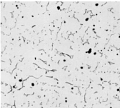
**Fig. 35** CF-16F alloy, a 25-mm (1-in.) bar, as-cast. The structure consists of selenide particles (black), precipitated carbide particles, and fine ferrite islands in a matrix of austenite. Dispersed selenide particles of this type improve the machining characteristics of the steel. Electrolytic: oxalic acid. 100×
