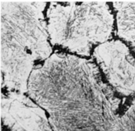
**Fig. 7** CA-15 alloy, 75-mm (3-in.) thick section, as-cast. Structure consists of islands of ferrite and dark-etching particles of chromium carbide at prior austenite grain boundaries in a matrix of martensite. See also [Fig. 8](#) and [9](#). Vilella's reagent. 200×
