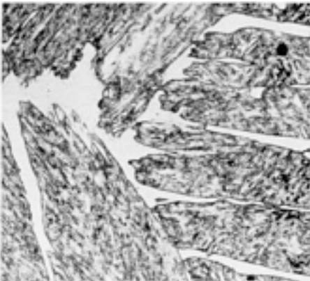
**Fig. 12** Same alloy and heat treatment as in [Fig. 10](#), but for a 150-mm (6-in.) thick section, showing the effect of section thickness on structure. Islands of ferrite appear in the matrix of tempered martensite. See also [Fig. 13](#). Vilella's reagent. 200×
