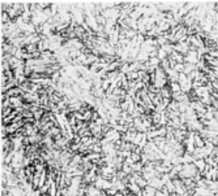
**Fig. 10** CA-15 alloy, 75-mm (3-in.) thick section, austenitized at 1010 °C (1850 °F), air cooled, tempered at 675 °C (1250 °F) for 4 h. The structure shows traces of ferrite in a matrix of tempered martensite. See also [Fig. 11](#). Vilella's reagent. 200×
