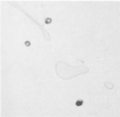
**Fig. 19** Same alloy and processing as [Fig. 18](#). Higher magnification of ferrite pools and inclusions in austenite matrix. Glyceregia. 1000×
