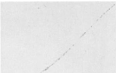
**Fig. 44** Same alloy and processing as [Fig. 43](#). Higher magnification of dispersed inclusions in austenite matrix. Electrolytic: oxalic acid. 1000×
