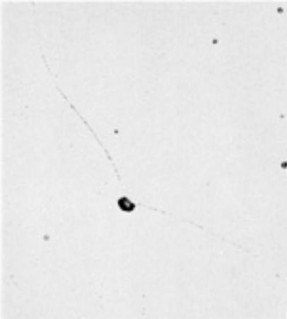
**Fig. 43** CN-7M alloy, solution treated 1 h at 1175 °C (2150 °F) and water quenched. Structure consists of austenite with dispersed inclusions. See also [Fig. 44](#). Electrolytic: oxalic acid. 400×
