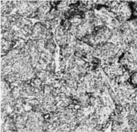
**Fig. 9** Same alloy and section thickness as for [Fig. 8](#), but heated to 1040 °C (1900 °F) and held for 3 h, air cooled, tempered at 690 °C (1275 °F) for 4 h. Ferrite islands have blended with the tempered martensite matrix. Ferric chloride. 100×
