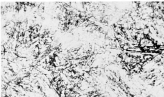
**Fig. 3** Same alloy and section thickness as for [Fig. 2](#), but heated to 1040 °C (1900 °F) and held 4 h, air cooled, tempered 5 h at 635 °C (1175 °F). The carbide particles at grain boundaries have dissolved during austenitizing; matrix consists of ferrite-free tempered martensite. Vilella's reagent. 500×
