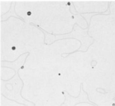
**Fig. 25** CF-8M alloy, solution treated 1 h at 1120 °C (2050 °F) and water quenched. Structure is austenite with ferrite and oxide inclusions. See also [Fig. 26](#). Kalling's reagent. 400×
