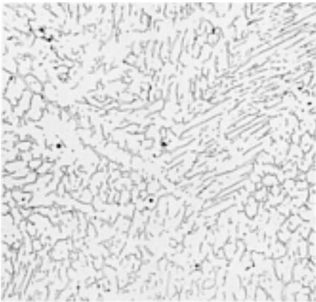
**Fig. 27** CF-8 alloy, 25-mm (1-in.) thick section, as sand cast. Structure contains 15 to 20% ferrite in an austenite matrix. [Fig. 28](#) shows the sand cast alloy after solution treatment; [Fig. 29](#) shows another as-cast structure. Electrolytic: oxalic acid. 80×
