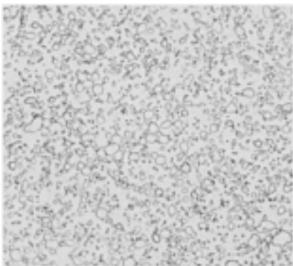
Fig. 32 AISI M2 molybdenum high-speed tool steel, spheroidize annealed. 4% picral. 1000×
