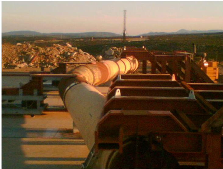
Fig.7a. View of Bend Testing Facility
