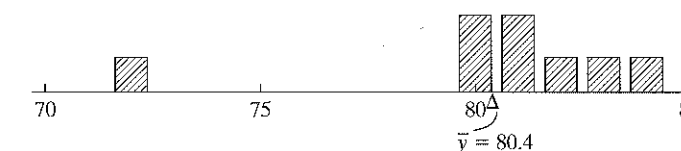
FIGURE 3.9: The Mean as the Center of Gravity, for Eastern Europe Data from Example 3.4. The line balances with a fulcrum at 80.4.
