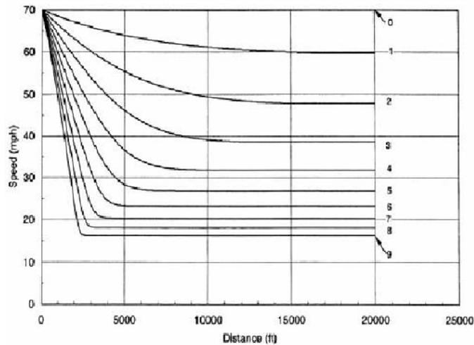
Exhibit 3-59. Speed-Distance Curves for a Typical Heavy Truck of 120 kg/kW [200 lb/hp] for Deceleration on Upgrades
