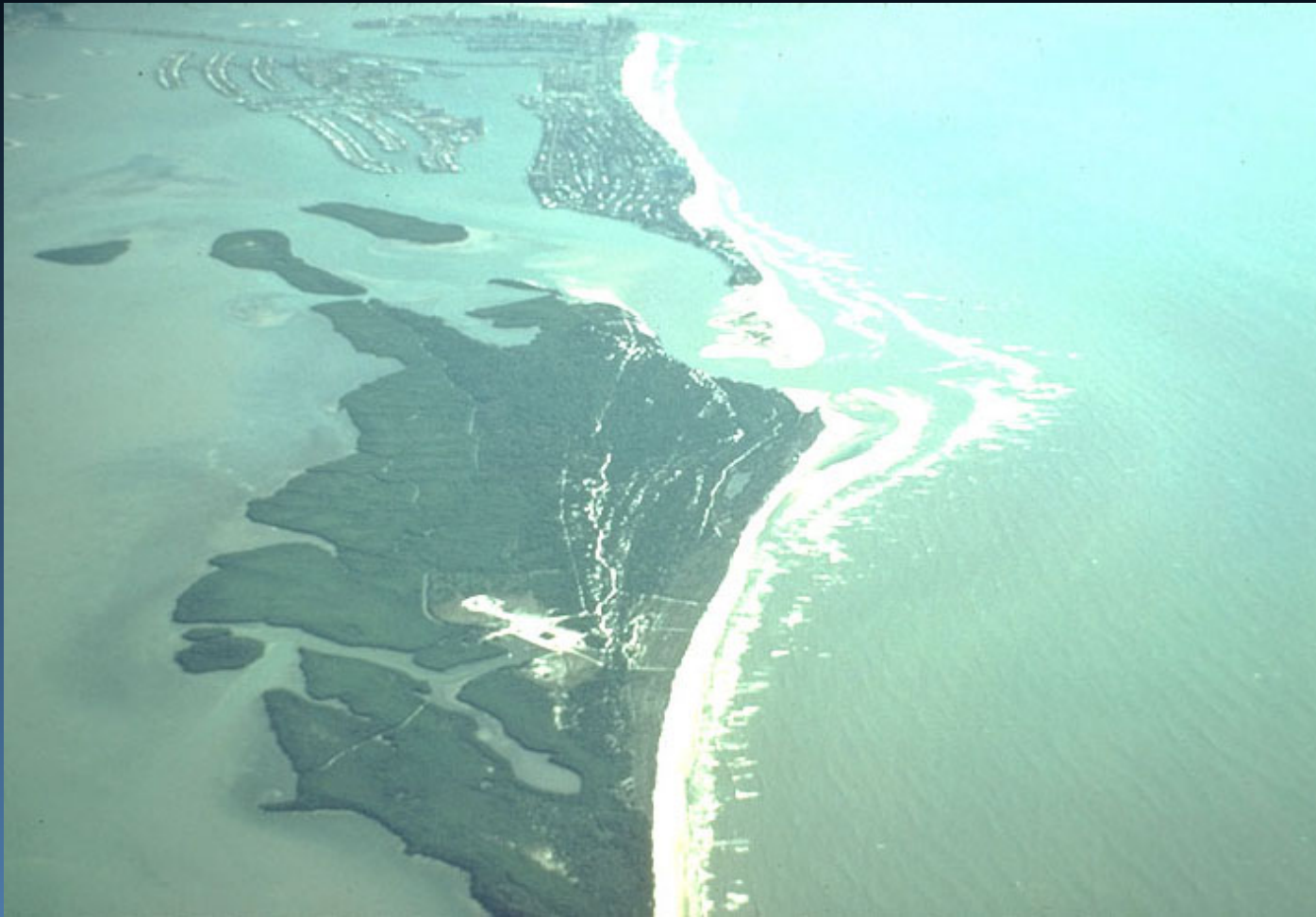
Waves breaking on an ebb-tidal delta formed at an inlet through a barrier island. Note beach ridges in vegetated area south of the inlet, associated with out-building of the barrier islands in the vicinity of the tidal delta. (Florida)
