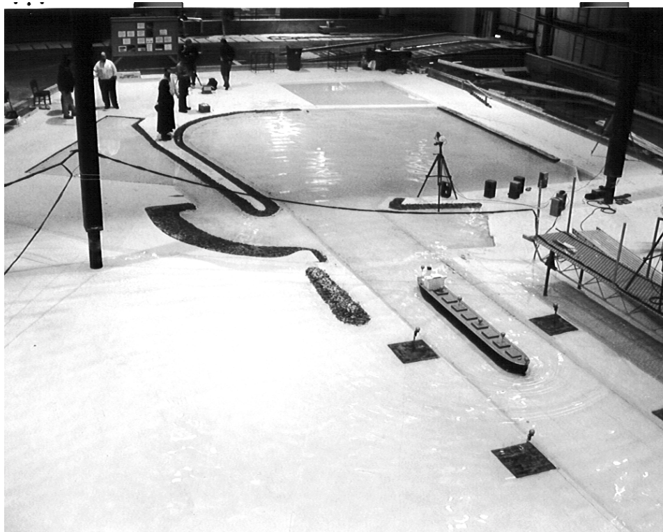
Figure V-5-57. Physical model of Barbers Point Harbor
