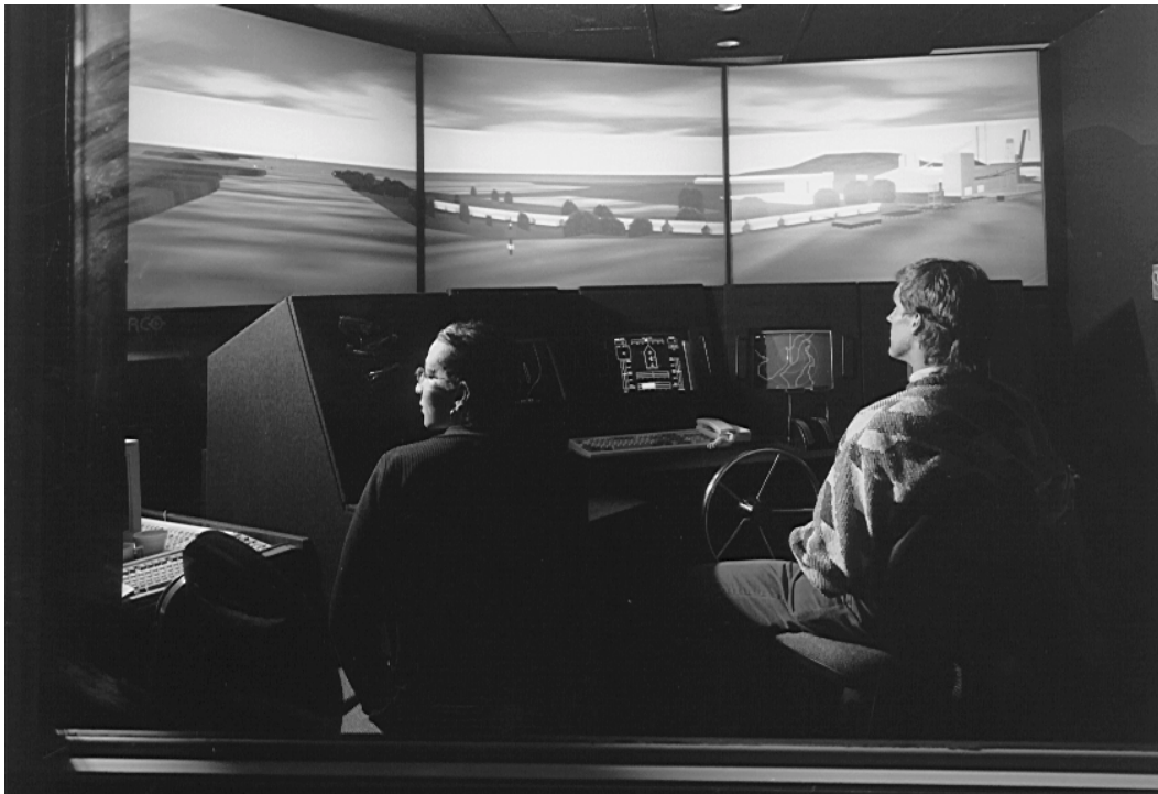
Figure V-5-66. Visual scene of Alafia River Harbor ship simulation study, inbound bulk carrier approaching dock
