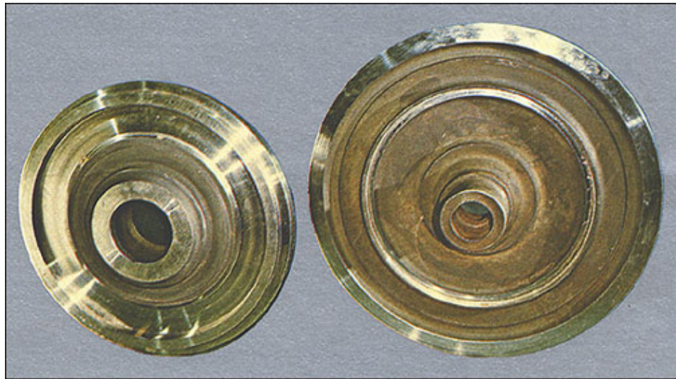
Discs for second stage for turbine aeroengines (HIP)
