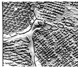
a. Cubical and Trigonal \gamma' in NASA IIb S-R Tested at 1900F (1040C) 2725X. Kent 15
