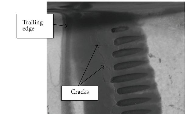
FIGURE 4: Cracks on the nozzle vane near the internal shroud close to the trailing edge.
