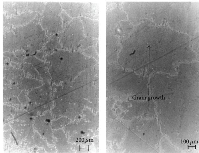
FIGURE 6: Grain growth in the high temperature (zone D).
