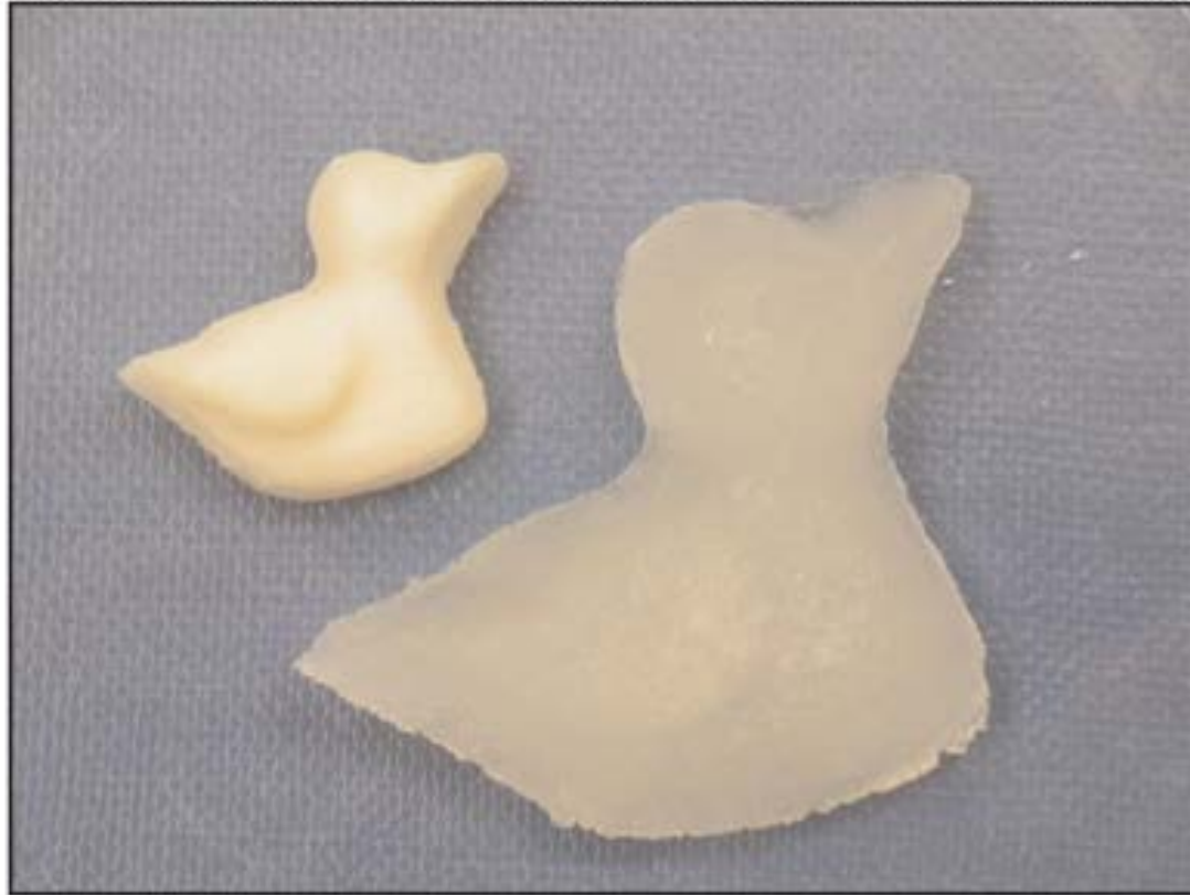
Swelling of a dried hydrogel (left) to a larger size of the same shape (right) in water.
